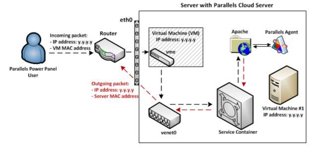
To avoid such problems, you can reconfigure the router to accept packets with the same IP address but different MAC addresses. You can also switch virtual machine's network adapter to the host-routed mode or create an additional network adapter and set it to work in the host-routed mode.
