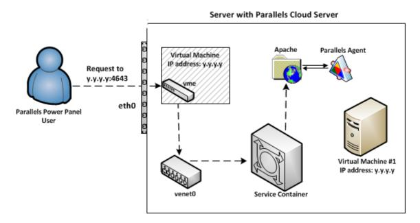
A data packet for a running virtual machine first arrives at its virtual interface (vme in the figure above) and only then is forwarded to venet0. The remaining steps are the same as those described for Containers and stopped virtual machines.
