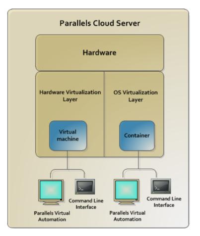
At the base resides server hardware. Next is the Parallels Cloud Server software which is installed directly on the server hardware and does not need any operating system for its functioning. Parallels Cloud Server includes two virtualization layers:
