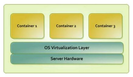
The OS virtualization layer ensures isolation and security of resources between different Containers. The virtualization layer makes each Container appear as a standalone server. Finally, the Container itself houses its own applications and workload. OS virtualization is streamlined for the best performance, management, and efficiency. Its main advantages are the following:
