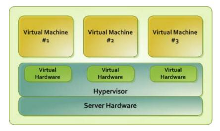
The following diagram shows the basic architecture of hardware virtualization.
