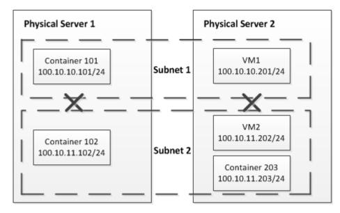
In this figure, the private network also includes two private subnets—Subnet 1 and Subnet 2, but the virtual machines and Containers included in these subnets reside on two physical servers. Container 101 and VM1 are joined to Subnet 1, and Container 102, Container 203, and VM2 are joined to Subnet 2. The virtual machine and Container on Subnet 1 can connect to each other but cannot access the virtual machines and Containers on Subnet 2, and vice versa.
